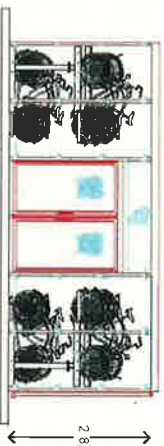
Supplier drawing showing the front elevation with 2 tier cycle storage along both sides of Hub
